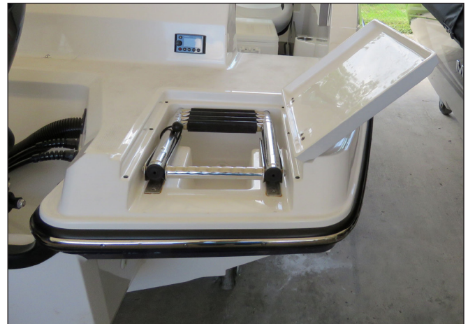
Boarding Ladder In Compartment
