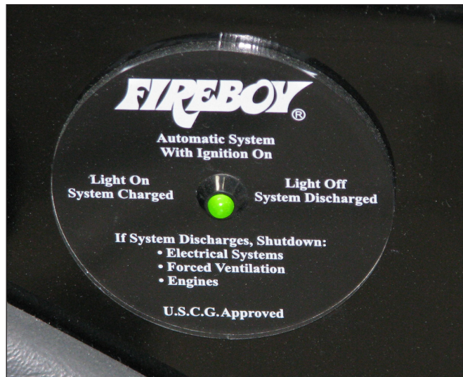
Typical Fire Extinguisher Panel In Helm
