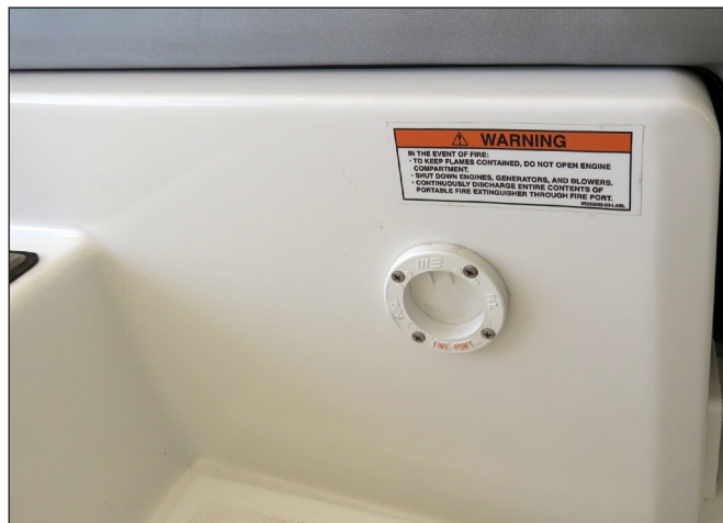
Typical Fire Port
