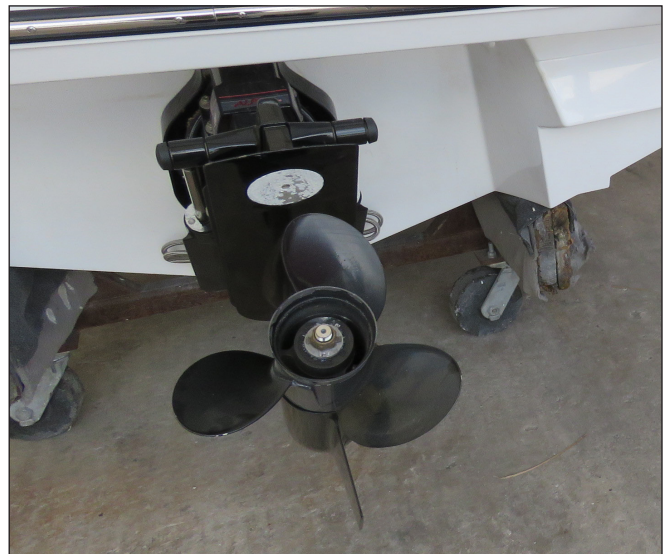
Typical Mercruiser Aluminum Propeller
