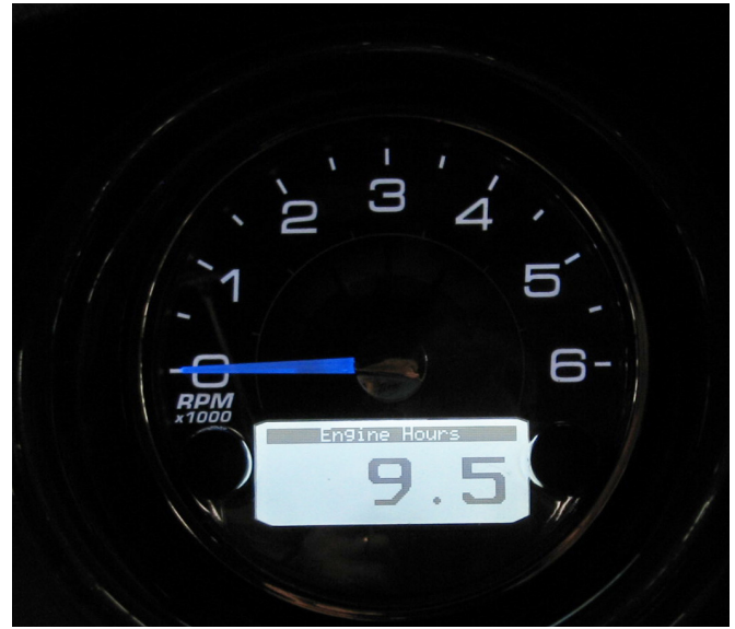
Digital LED Display Screen In Tachometer
