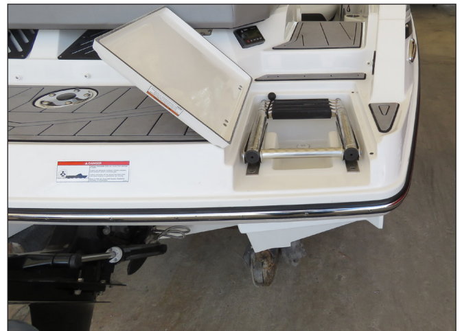
Boarding Ladder In Compartment
