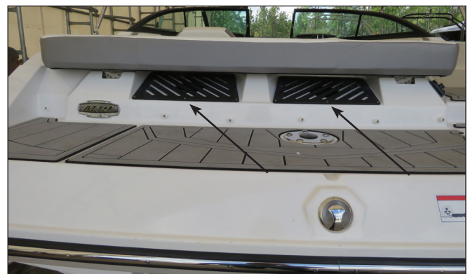
Engine Compartment Vents
