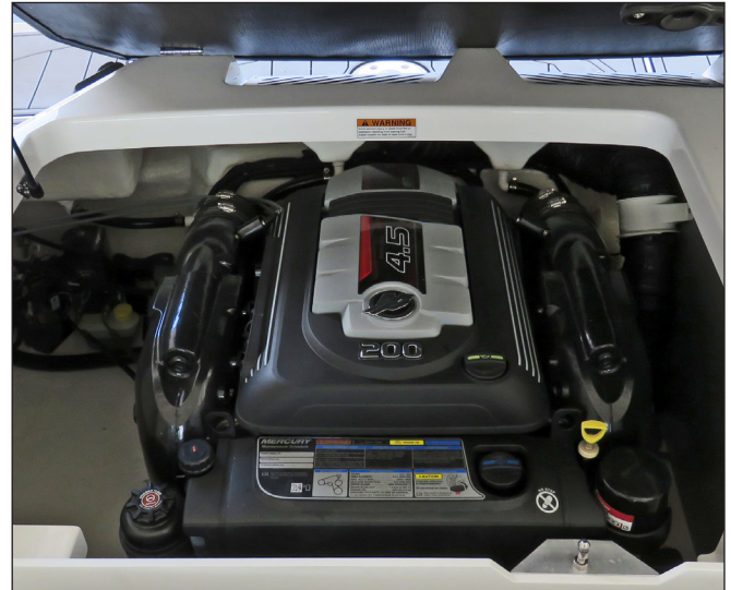
Typical Mercruiser Gas Engine
