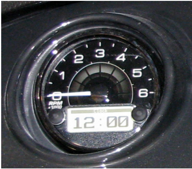
Digital LED Display Screen In Tachometer
