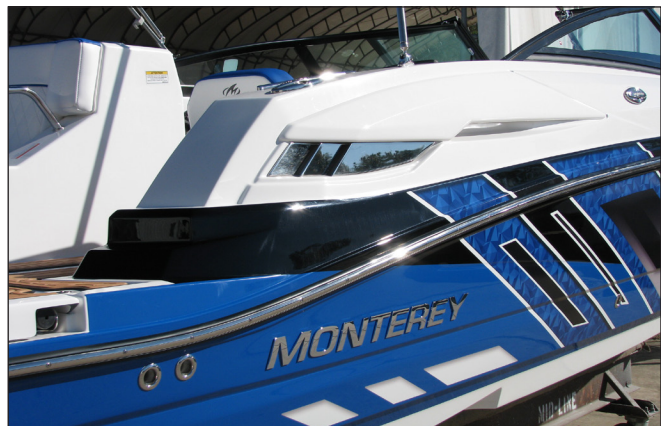
Bilge Compartment Vents
