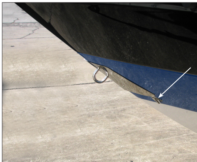
Rope Locker Drain
