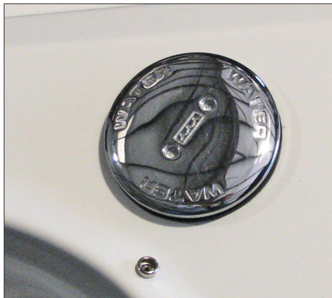
Fresh Water Fill
