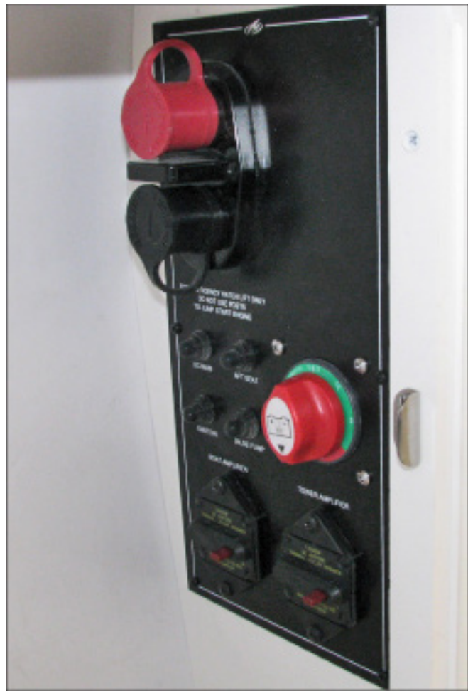
Dual Battery Switch Panel w/ Circuit Breakers, Engine Hatch Jumper Terminals & Sound System Amplifiers
