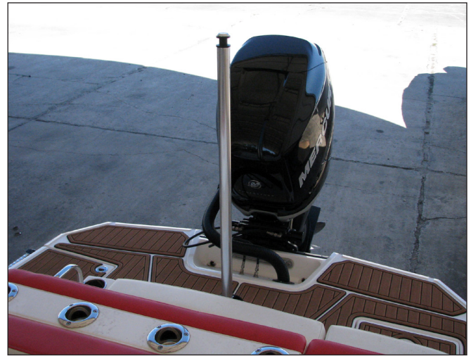
Ski Tow Pylon
