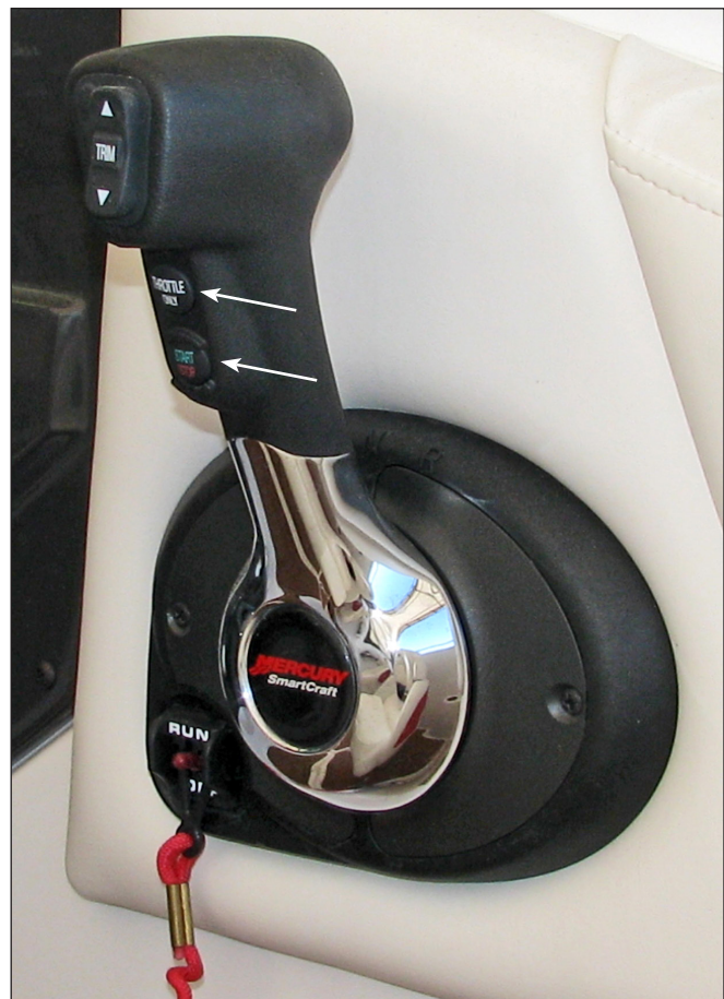
Typical Mercury Electronic Control & Switches
