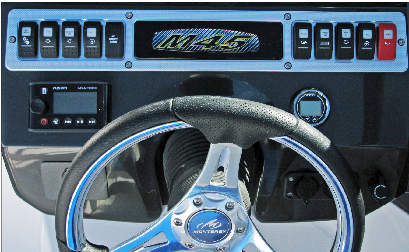
Helm Switch Panels
