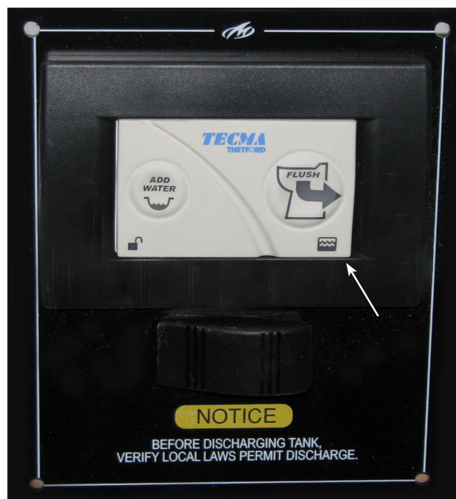
Head Compartment Toilet Control Panel
