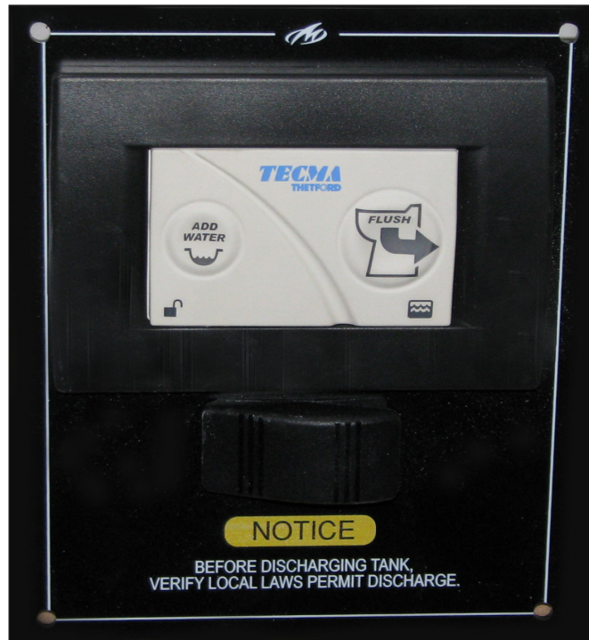
Electric Head Control Panel In Head Compartment
