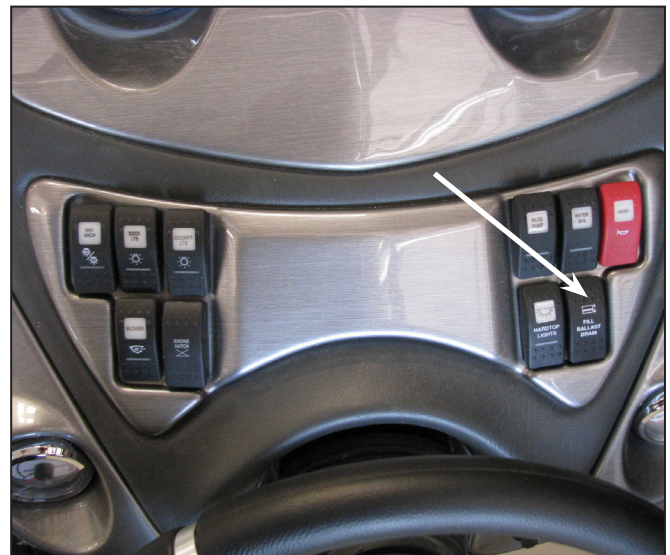
Ballast Tank Pump Control Switch
