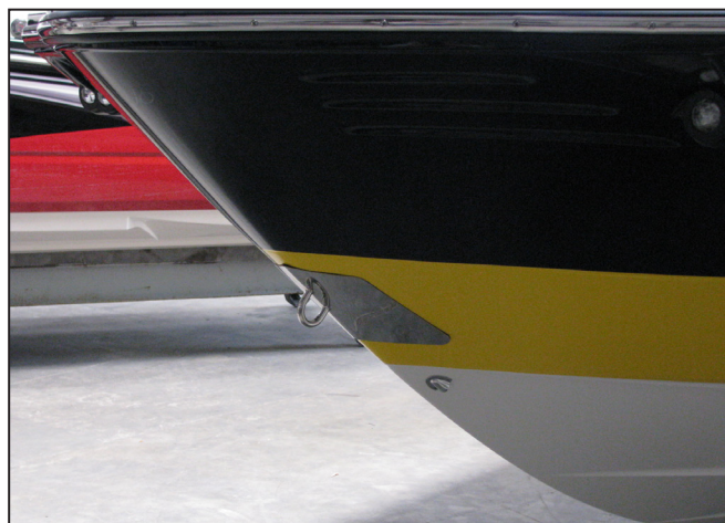
Rope Locker Drain
