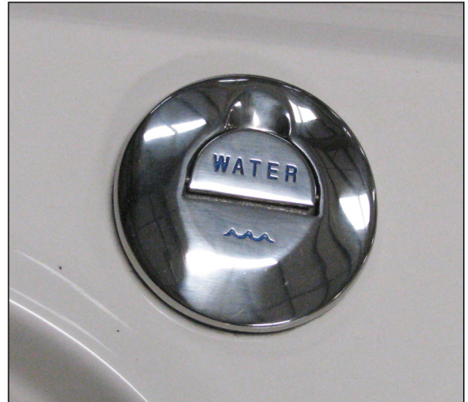
Fresh Water Fill
