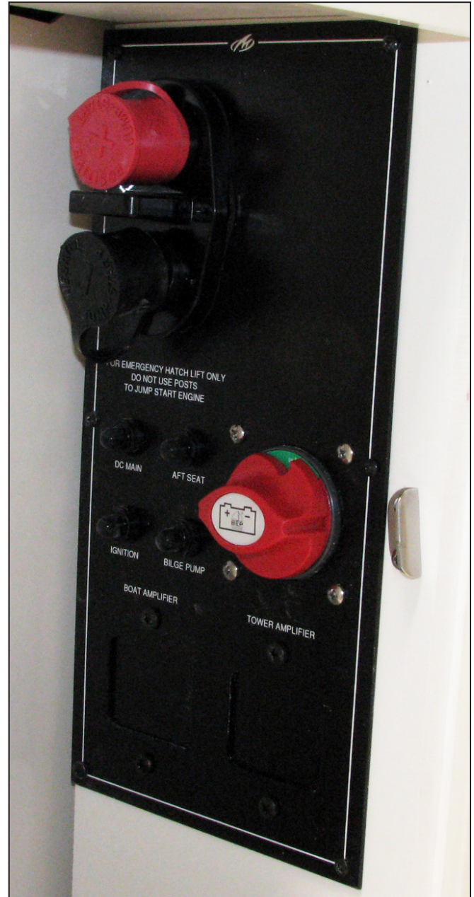
M4 Single Battery Switch Panel with Circuit Breakers and Engine Hatch Battery Jumper Terminals
