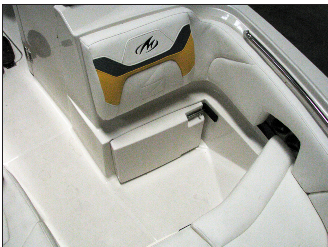
M4 with Bow Lounge Seat Cushion Removed and Foldout Support Latched in the Stored Position
