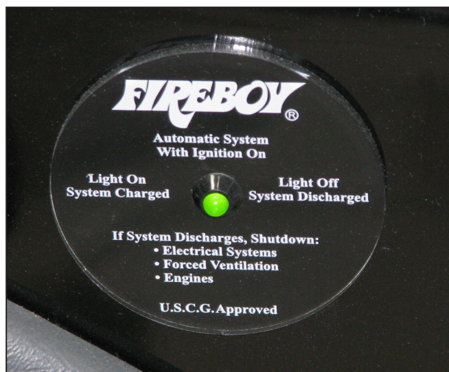
Fire Extinguisher Panel in Helm
