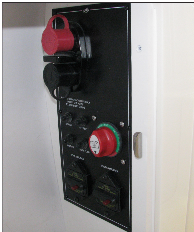
MSX Dual Battery Switch Panel w/ Circuit Breakers, Engine Hatch Jumper Terminals and Sound System Amplifiers
