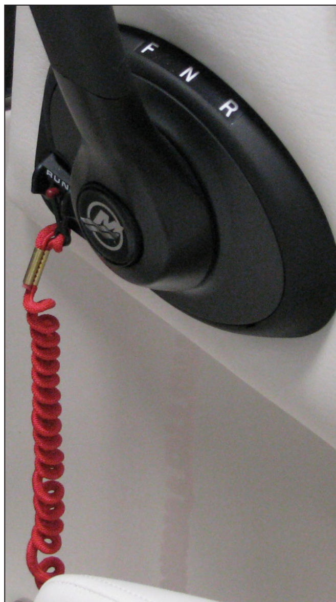
Mercruiser Control Emergency Stop Switch and Lanyard
