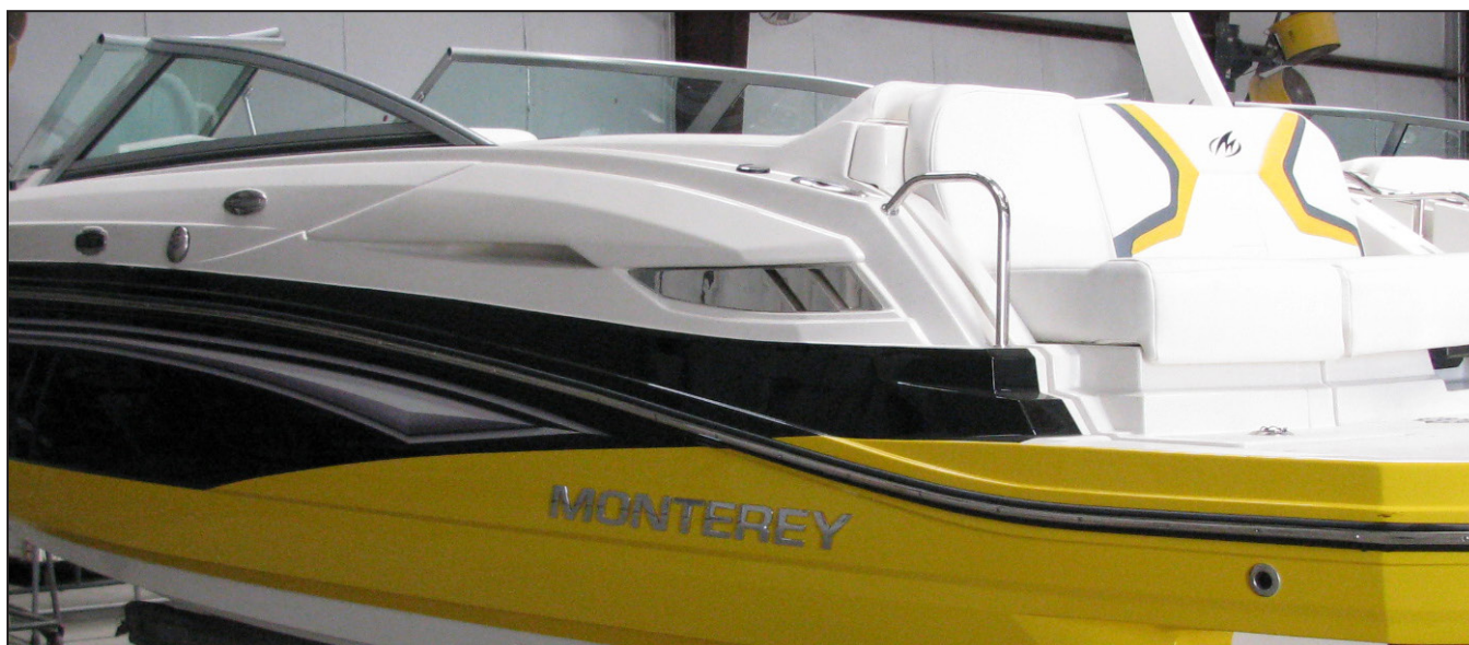
Port Side Engine Compartment Vent
