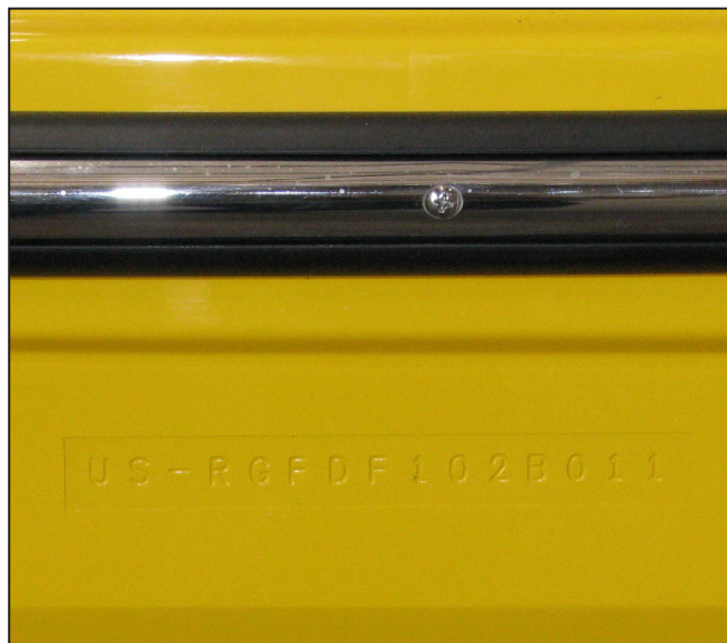
Hull ID # On Starboard Side of Transom
