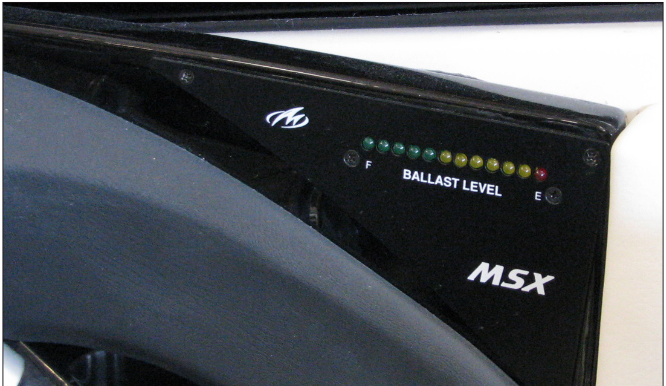
Ballast Tank Level Indicator
