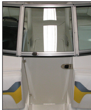
Outer Door Latched to Close Off Bow Area Walk-Thru
