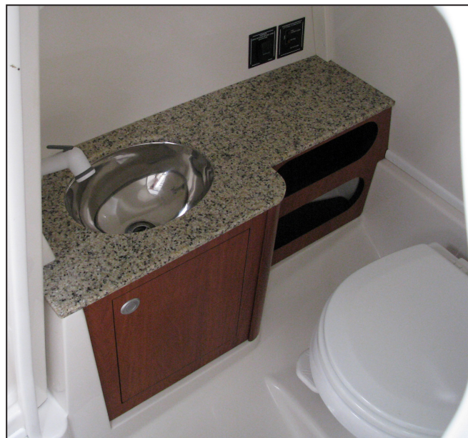
M6 Head Compartment and Vacuflush Marine Toilet
