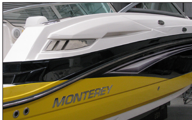
Starboard Engine Compartment Vent
