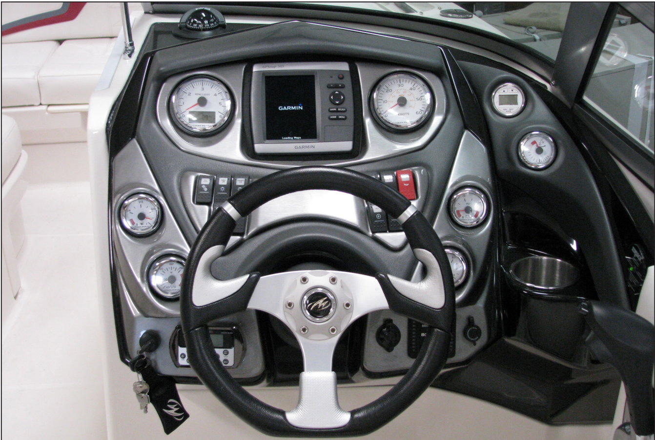
Standard Speedometer and Tachometer with Hour Meter
