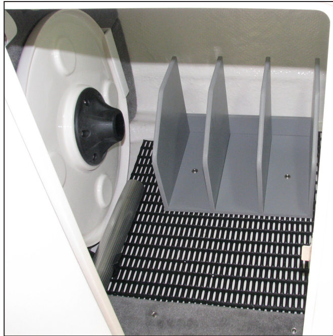
Helm Storage Compartment w/ table and Cushion Brackets
