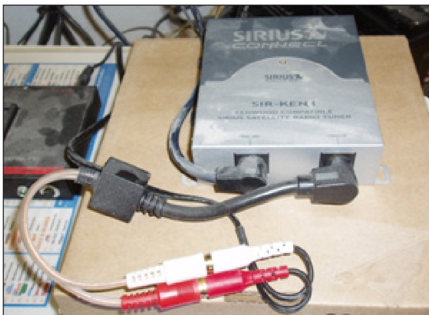
MP3 ADAPTER CONNECTION IF SIRIUS RADIO INSTALLED, PLUG ADAPTER INTO SIRIUS MODULE
