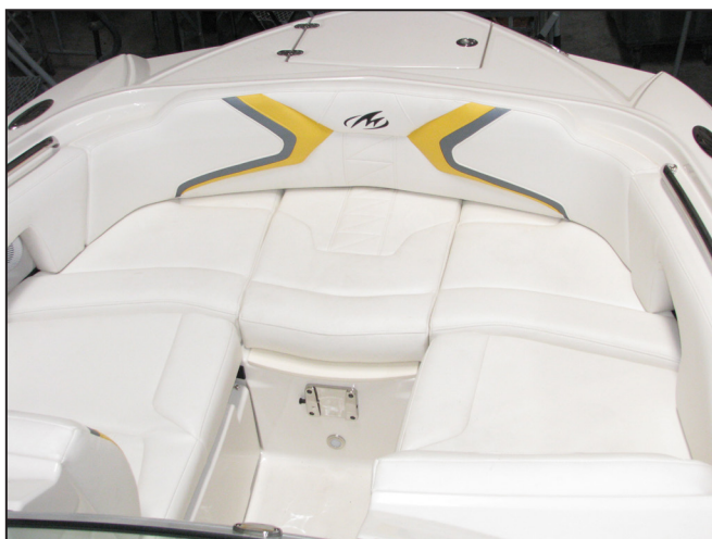
M4 Bow Seat Area with Lounge Seat Insert Cushions and Cockpit Table Mounting Bracket
