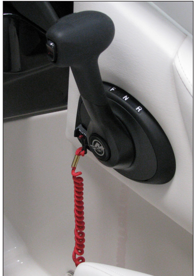
Mercruiser Side Mount Control and Stop Switch
