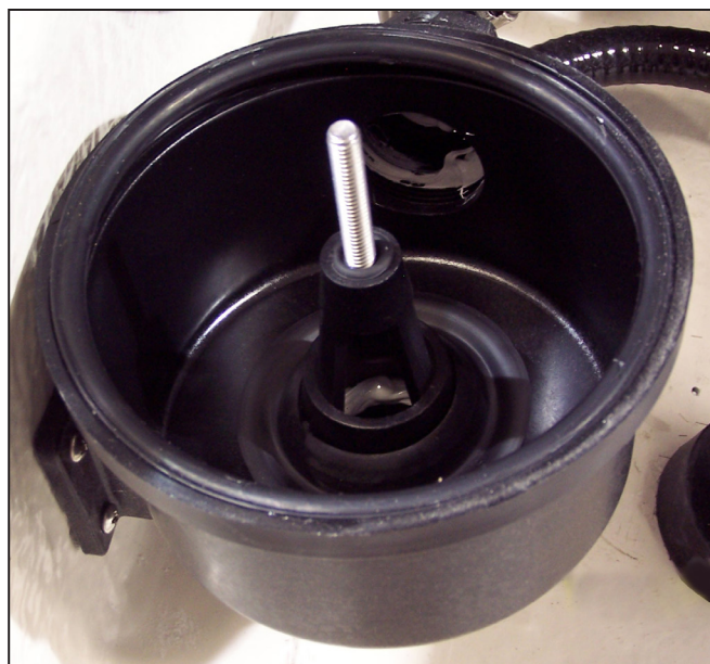
Sea Strainer with Basket Removed
