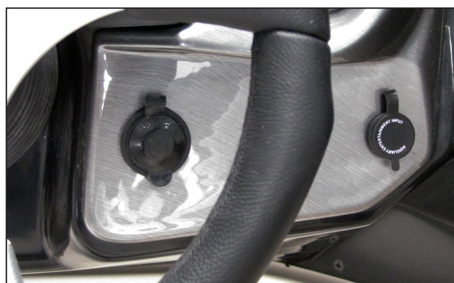
12-Volt Accessory Receptacle and MP3 Connection
