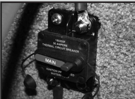
Main Dash Power-Circuit Breaker
