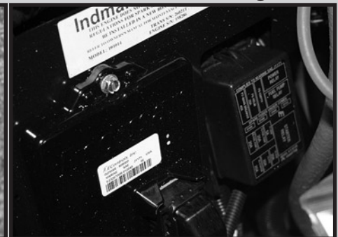
Fuse Panel - Back of Engine
