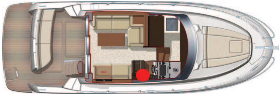
Extinguisher remote control
