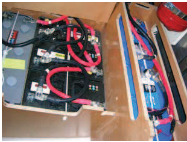
Set Batteries - Engines : 2 x 75A Service : 3 x 110A Power : 1 x 140A Engine compartment
