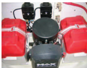
Set Batteries - Bow thruster : 2 x 50A Forward cabin
