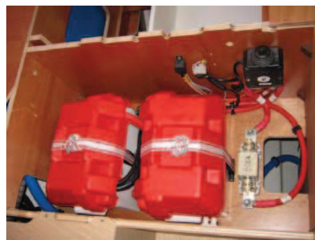
Service batteries: 3 x 80A Spare service batteries: 1 x 80A
