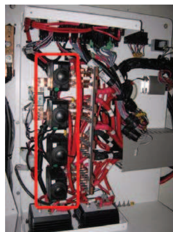
Location - Battery switch: Engine compartment
