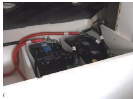
Propeller battery: 2 x 50A
