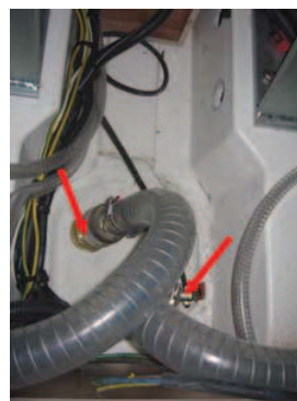
Sea water inlet valve for engine
