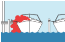
Blocked exhaust outlets.
