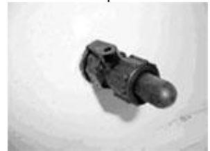
Lever on the aerator fitting is open
