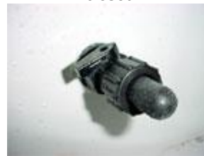
Lever on the aerator fitting is closed
