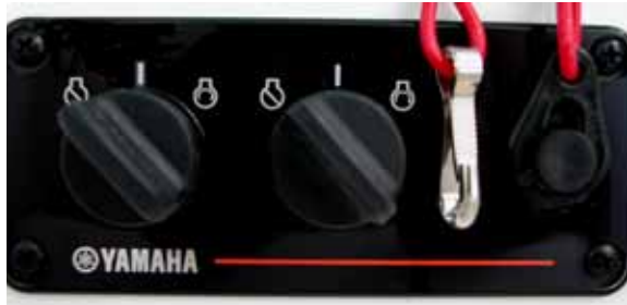
Engine Stop Switch
