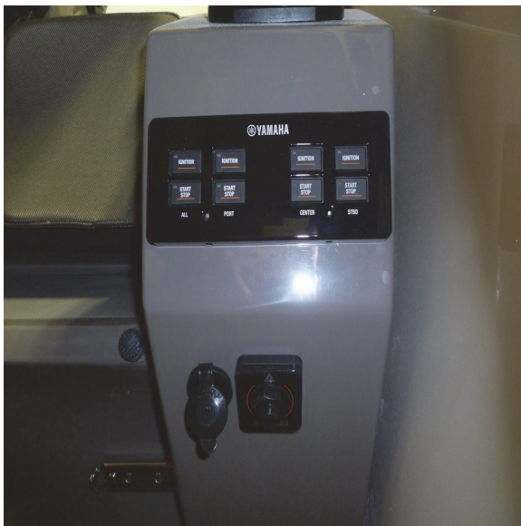
Start Stop Switch Panel
