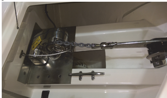
Anchor Line Secured Using Cable
