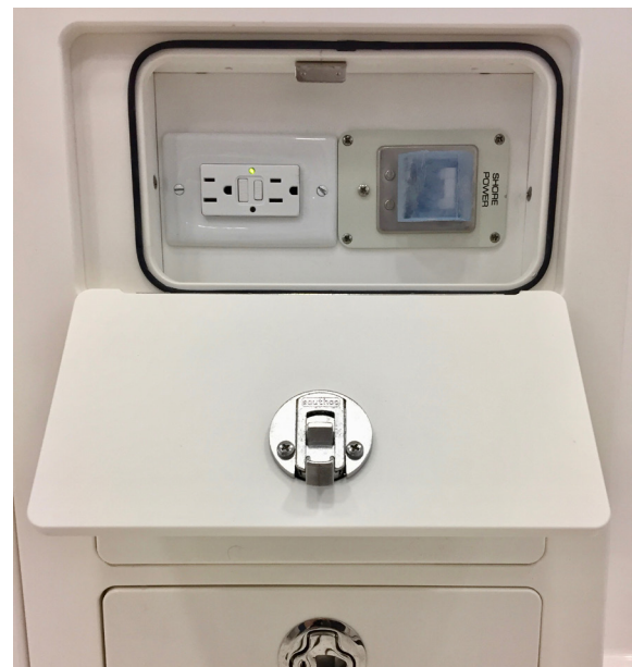
Main shore power breaker and outlet in aft cockpit power cabinet
