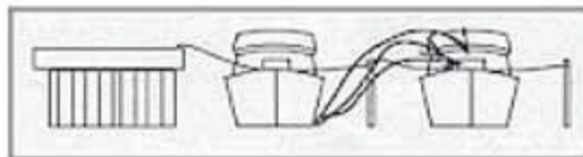
NEARBY BOAT GENERATOR EXHAUST
