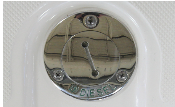
Diesel Fuel Fill
