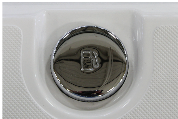
Gasoline Fuel Fill
