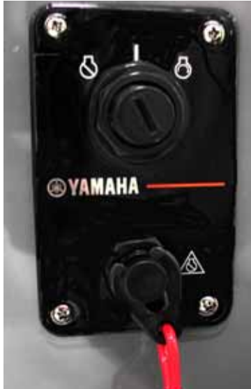
Engine Stop Switch
