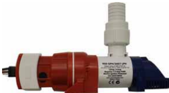
Aft Automatic Bilge Pump
