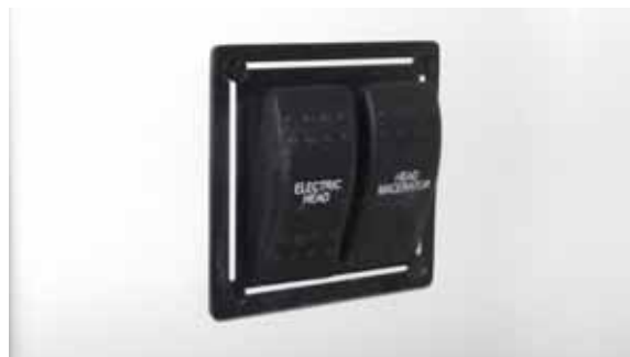
Head Macerator Switch
