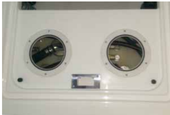
Gas Tank Valves
