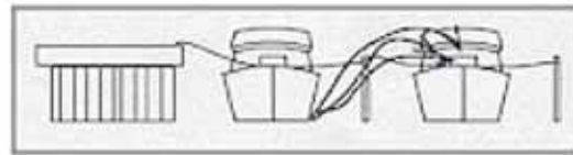
NEARBY BOAT GENERATOR EXHAUST
