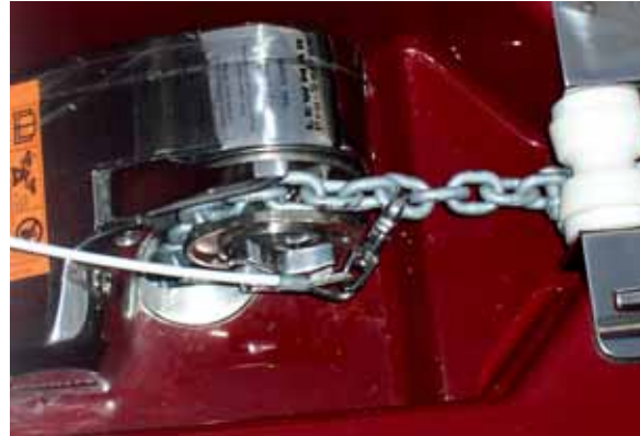
Anchor Chain Secured
