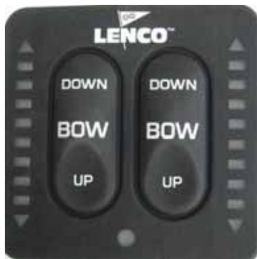
Trim Tab Switches
