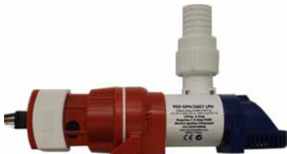
Aft Automatic Bilge Pump
