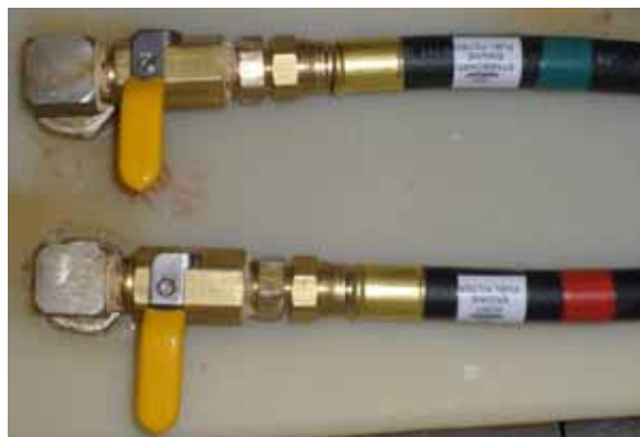
Fuel Tank Shut Off Valves
