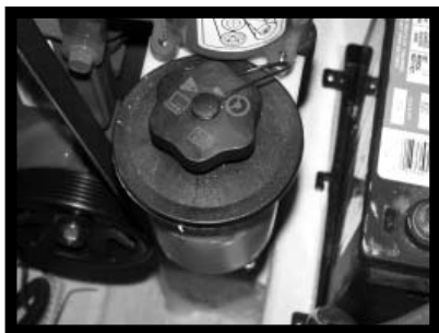
Typical Volvo Power Steering Fluid Fill Typical Mercury Power Steering Fluid Fill
