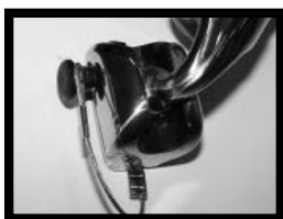
Typical Saddle Joint
