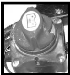
Typical Two Position Battery Switch
