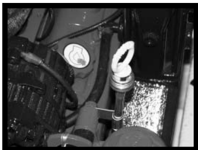
Typical Volvo Engine Oil Dipstick And Fill Typical Mercury Engine Oil Dipstick
