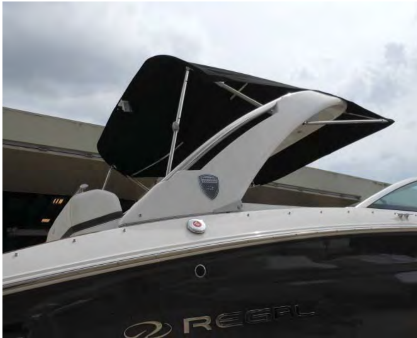
Q. COMPLETED BIMINI TOP ASSEMBLY.
