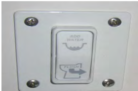
TYPICAL HEAD WALL SWITCH
