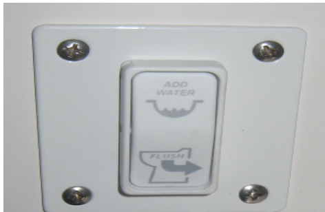
TYPICAL HEAD WALL SWITCH
