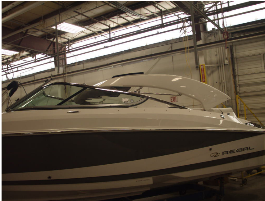
Typical Power Tower Shown In (Bridge) Full Forward Position
