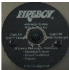
Typical Dashboard Automatic Extinguishing System Light
