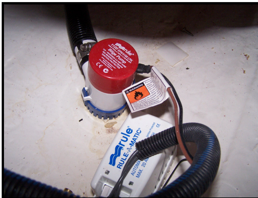
Typical Bilge Pump And Automatic Float Switch
