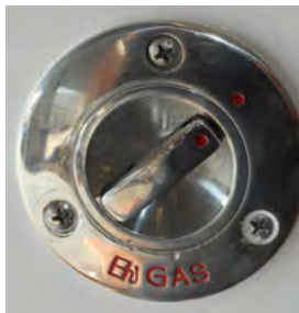
COMBO FUEL FILL/ INTERNAL VENT
