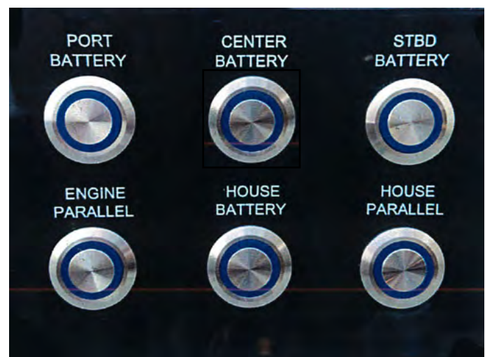
TYPICAL BATTERY ACTIVATION PANEL
