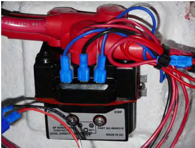
WINDLASS DUAL DIRECTION SOLENOID SWITCH
