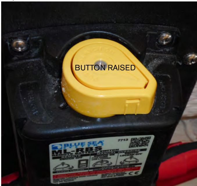
REMOTE BATTERY SWITCH LOCKED -OFF POSITION
