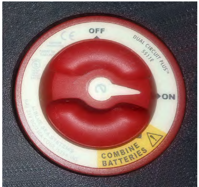
TYPICAL DUAL BATTERY SWITCH
