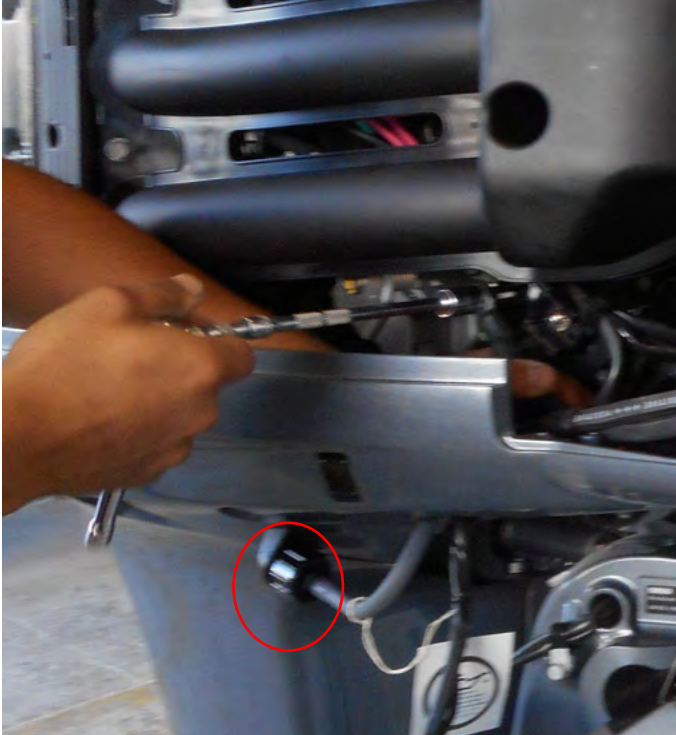
SEE FLUSHING DEVICE ABOVE CIRCLED
