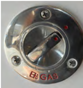
COMBO FUEL FILL/ INTERNAL VENT
