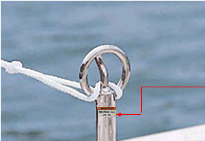
TYPICAL WATER SPORTS OUTBOARD PYLON
