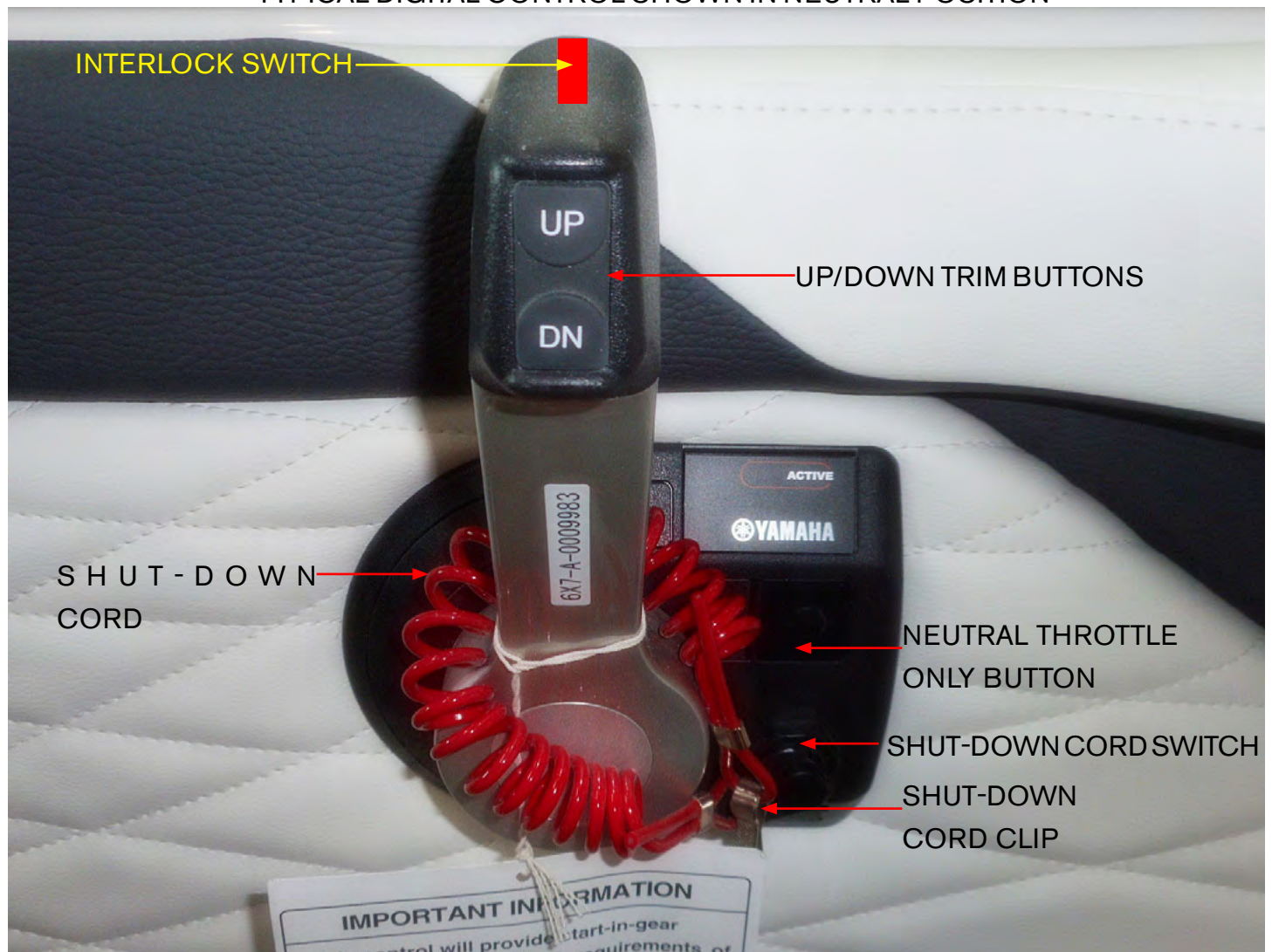
TYPICAL DIGITAL CONTROL SHOWN IN NEUTRAL POSITION
