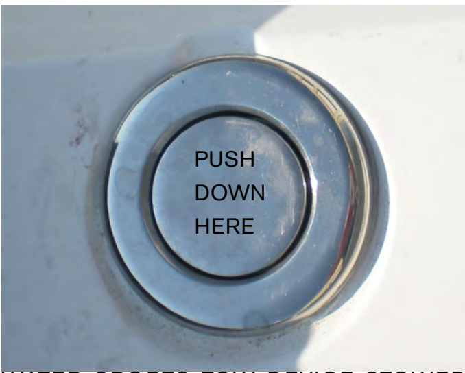
WATER SPORTS TOW DEVICE-STOWED POSITION
