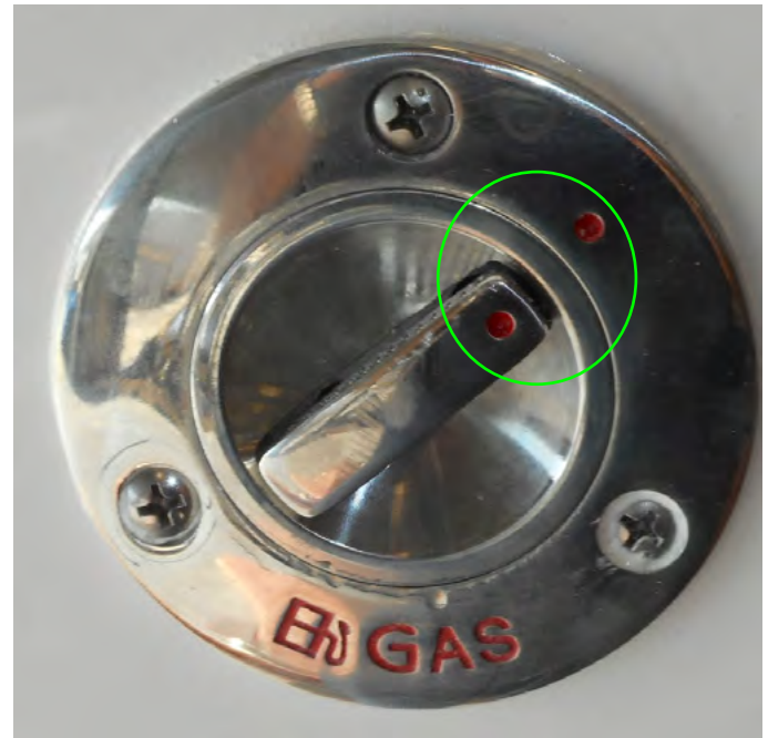
FUEL FILL CLOSED AND POINTS LINED UP
