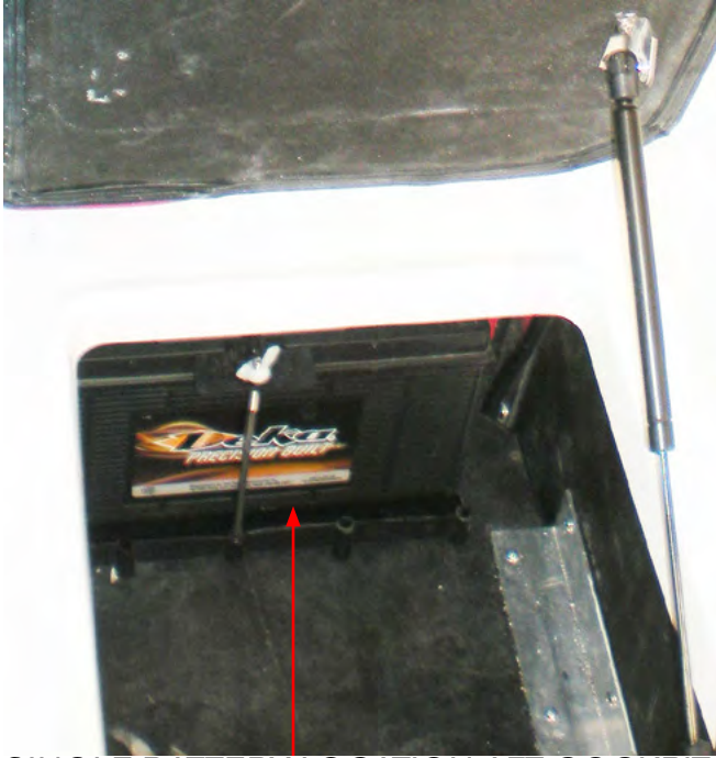
SINGLE BATTERY LOCATION AFT COCKPIT
