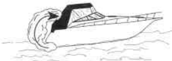
FIGURE 2.3 CO ACCUMULATION WITH PROTECTIVE COVERINGS
