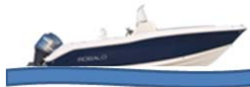
Incorrect Causes boat to "porpoise"
