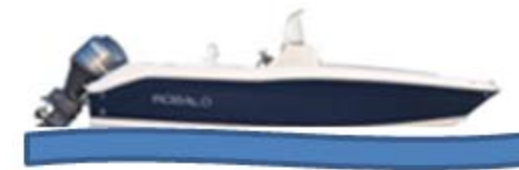
Incorrect Causes boat to "plow"
