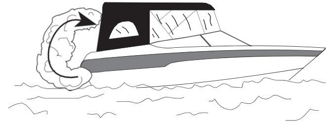
Figure 2.3 - Exhaust accumulations while canvas is in place
