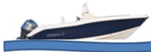
Incorrect Causes boat to "porpoise"
