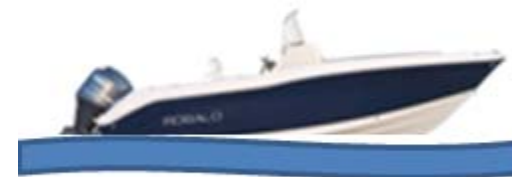
Incorrect Causes boat to "porpoise"
