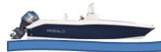
Incorrect Causes boat to "plow"
