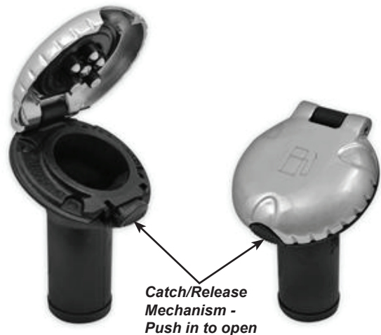
Figure B26: Fuel Deck Fill Catch/Release Mechanism
