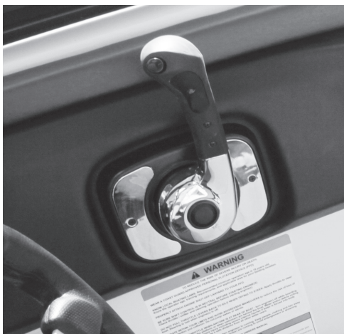
Figure D2: Throttle Control in Neutral Position
