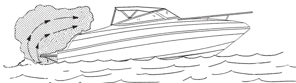
Figure A13: Exhaust Gas Accumulation at Swim Platform
