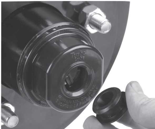
Figure F18: Turbo Lube Hub - Front Fill Model
