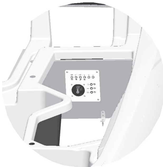
Figure B10: Battery Switch Panel Location
