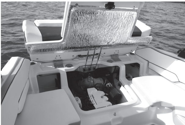
Figure C33: Raised Center Stern Seat - Engine Compartment Access
