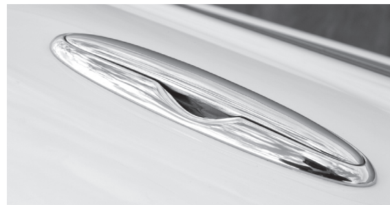
Figure C3: Pull-Up Cleat - Retracted
