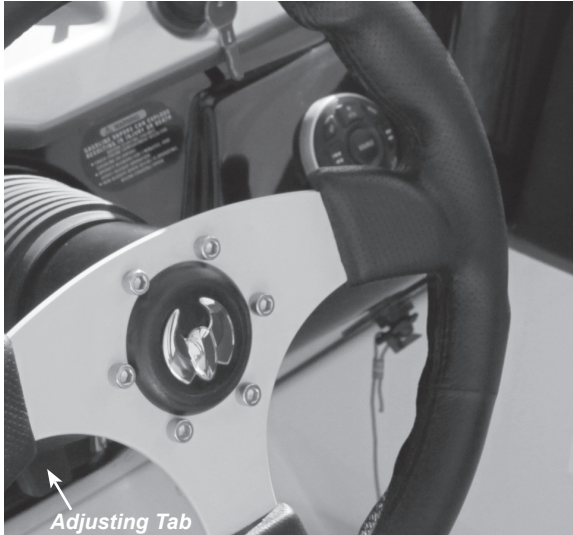
Figure B5: Tilt Steering Wheel (Adjusting Tab)
