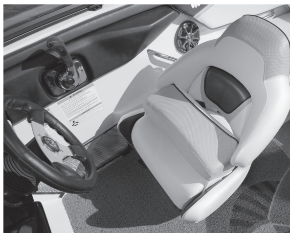
Figure C24: Bucket Seat with Flip-Up Bolster (Up)
