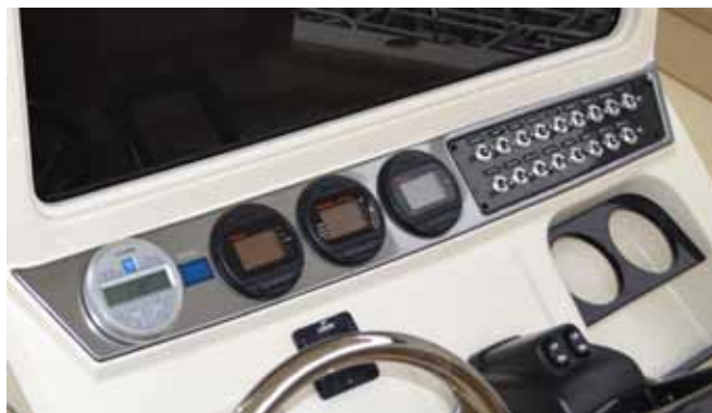
Helm Gauges and Switch Panel
