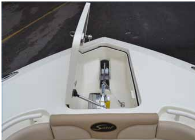
Anchor Locker Deck Hatch
