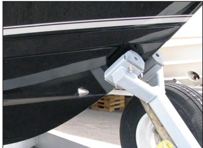
Rope Locker Drain
