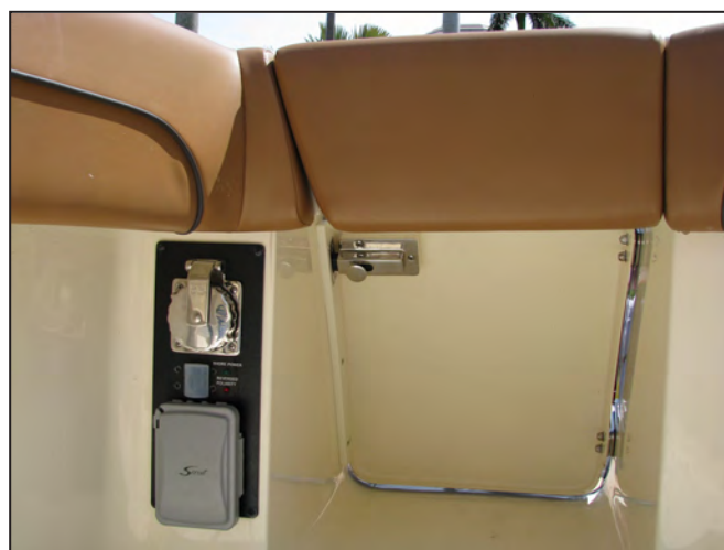
Shore Power Inlet, Transom Door and Gate
