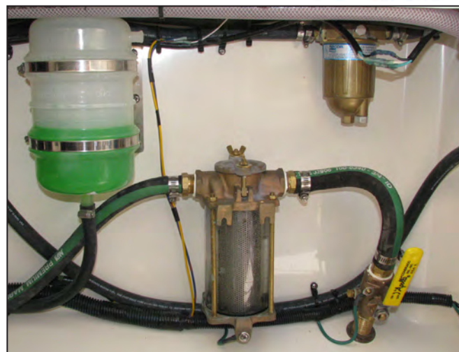
Primary Generator Diesel Fuel Filter, Coolant Recovery Tank, Sea Strainer and Intake Valve
