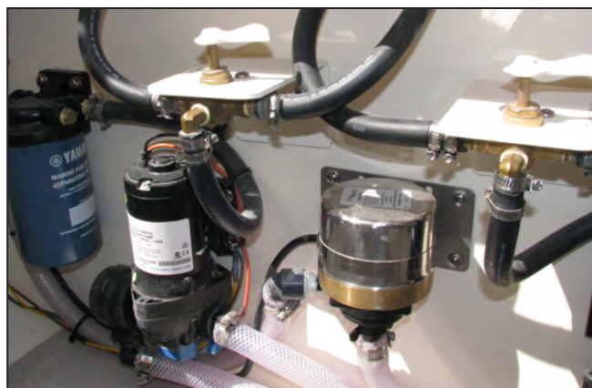
Raw Water Washdown and Air Conditioning/Freezer Circulating Pump
