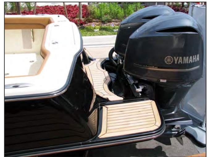
Engine Mounting System and Swim Platform
