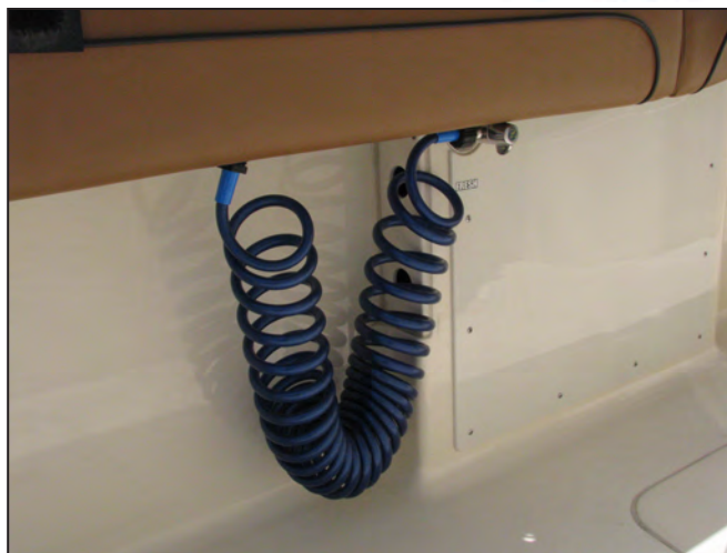
Cockpit Fresh Water Washdown Hose and Faucet
