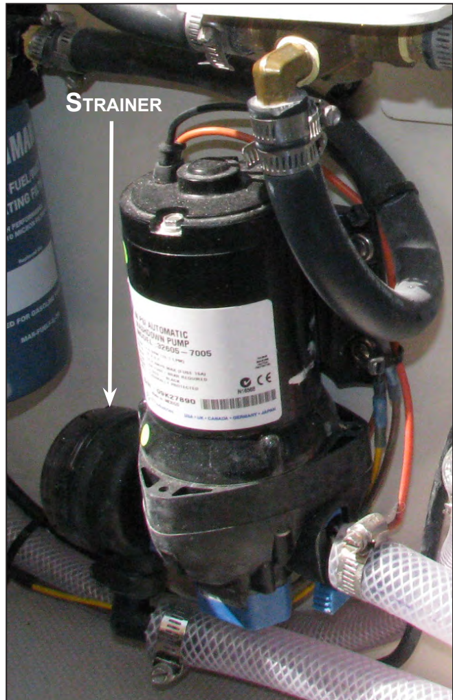
Raw Water Washdown Pump and Strainer
