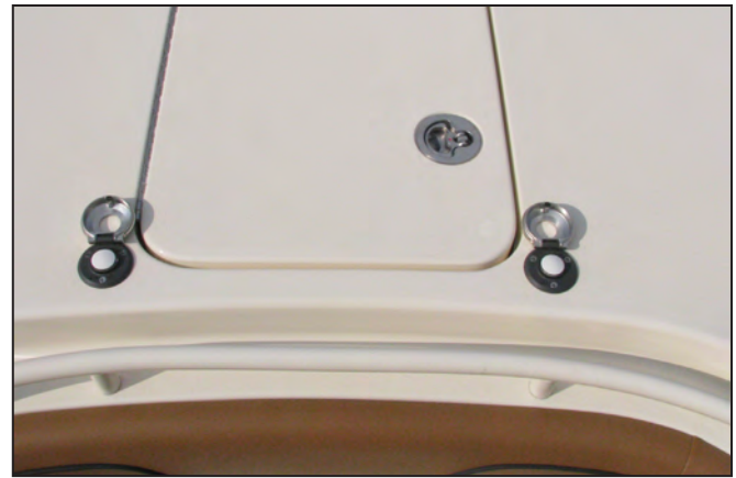
Windlass Foot Switches and Safety Covers
