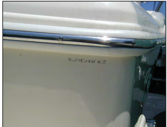
Hull ID Number on Starboard Transom
