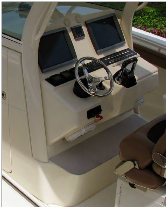
Helm, Controls, Switch Panels and Electronics
