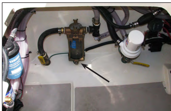
Seawater Intake Strainer for the Air Conditioning/Freezer Circulating and Raw Water Washdown Pumps
