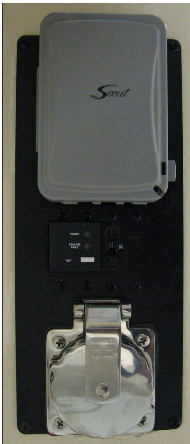
Boat AC Inlet, Main Circuit Breaker and ELCI Power Available Light and AC GFI Outlet
