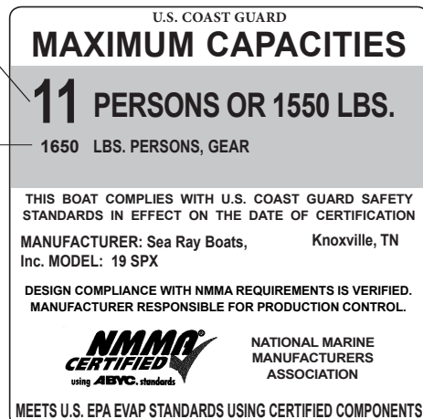
CAPACITY PLATE (INTERNATIONAL CERTIFICATION) (FIG. 2.1)
