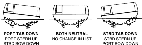
EFFECTS OF PORT AND STBD TRIM TAB ADJUSTMENT
