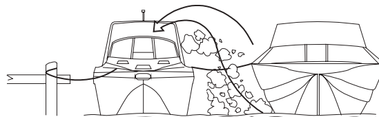
OPERATING ENGINE AND/OR GENERATOR IN CONFINED SPACES.
