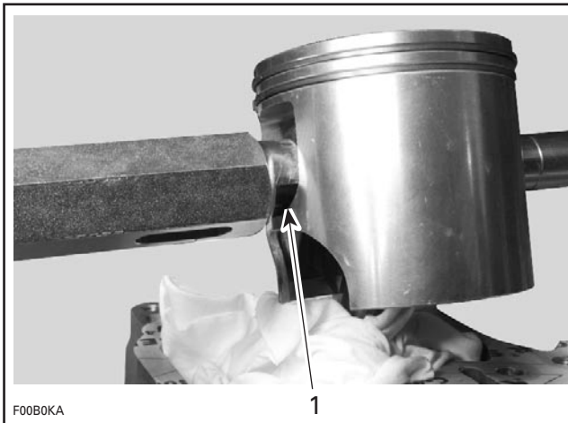
1. Tool cut-out toward bottom of piston
