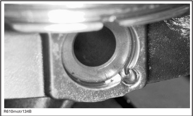
CORRECT POSITION OF THE PISTON CIRCLIP
