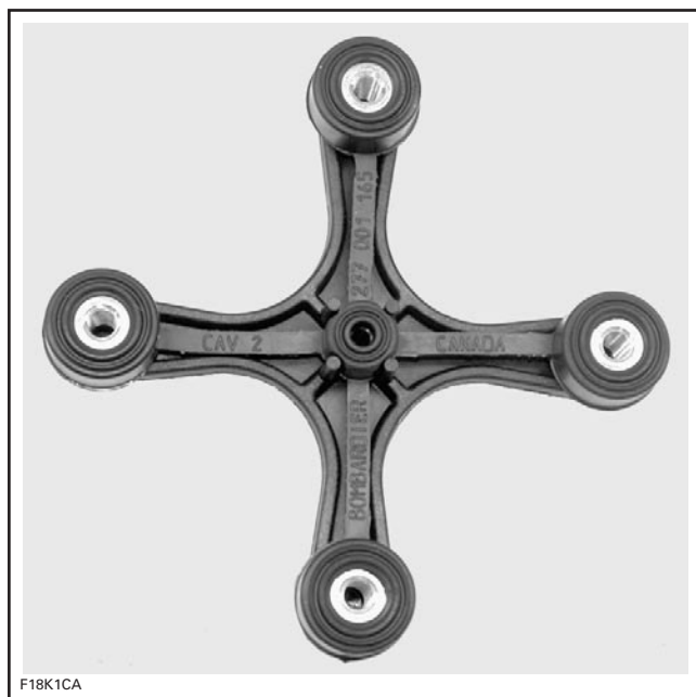
GASKET INSTALLED ON SUPPORT PLATE
