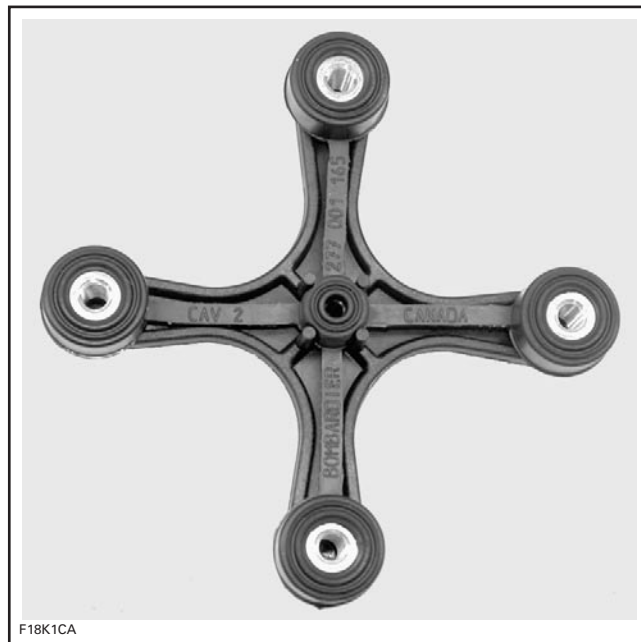
GASKET INSTALLED ON SUPPORT PLATE
