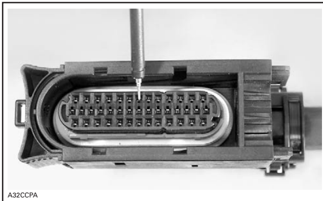
PROBE ONLY TOP OF TERMINAL
