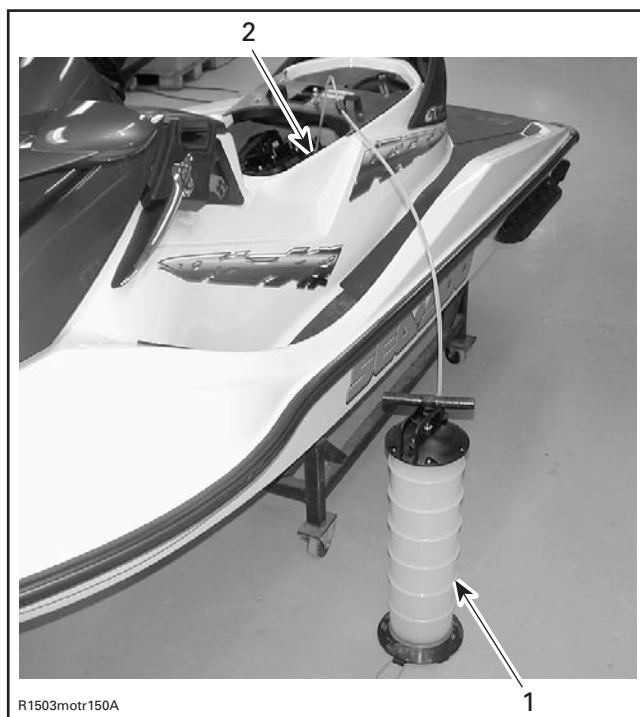
1. Suction pump 2. Siphon tube in dipstick hole
