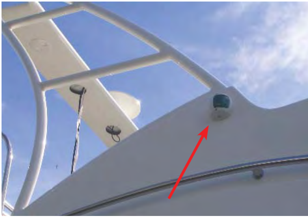
The Starboard Navigation Light is GREEN.
