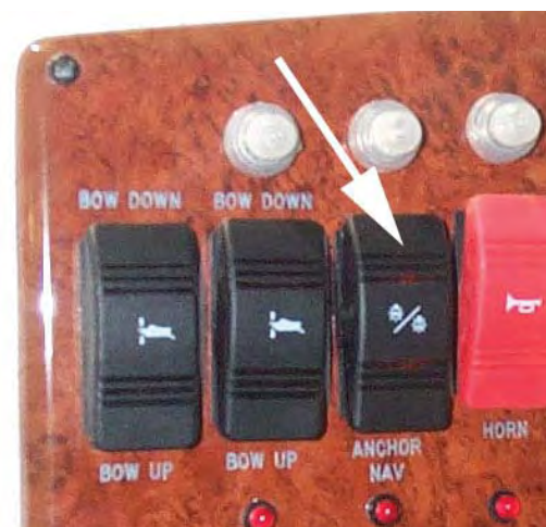
The Navigation/Anchor Light switch is located at the helm station.
