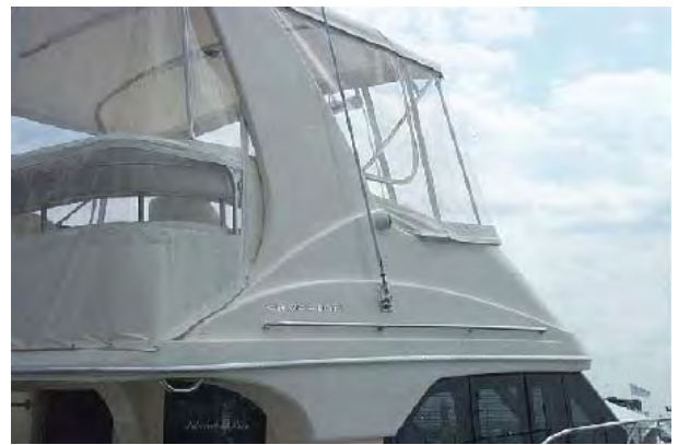
The Starboard Navigation Light is GREEN.
