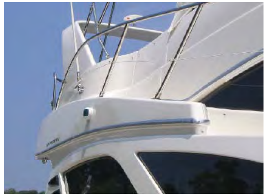
The Starboard Navigation Light is GREEN.
