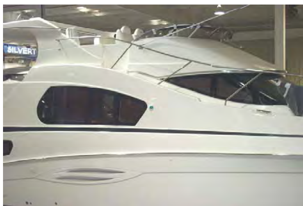
The Starboard Navigation Light is GREEN.
