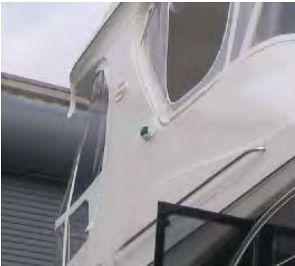
The Starboard Navigation Light is GREEN.
