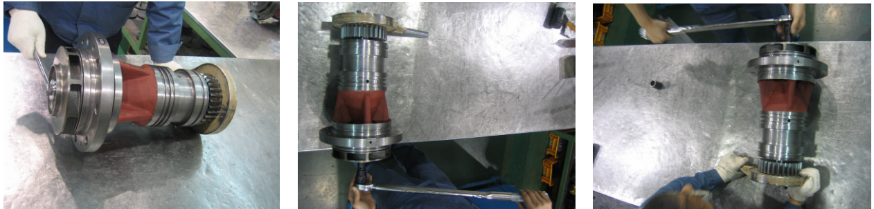
Fig.10 Tightening impeller by torque 120Nm (임펠러 조임)
