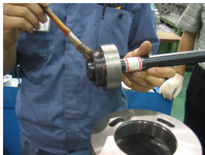
Fig.2 Assembly of oil seal (오일씰 조립 방법)
