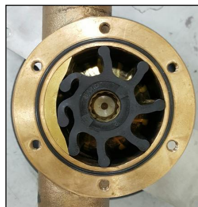
<Seawater pump & Impeller>
