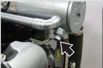
MV10 Heat Exchanger Anode (one each port and starboard)
