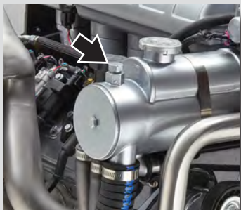
MV8-570 Heat Exchanger Anode
