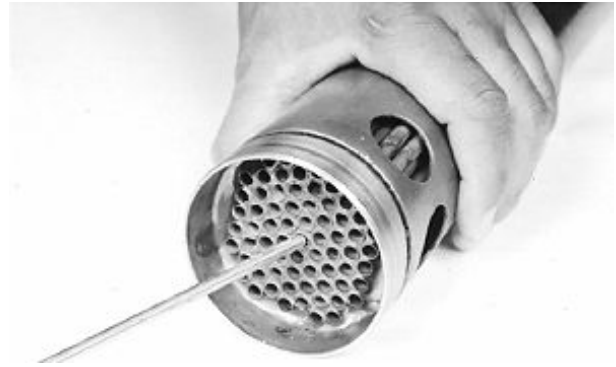
Clean Heat Exchanger
