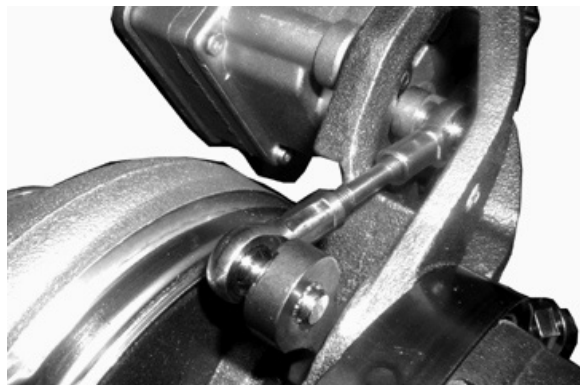
Actuator Linkage (Earlier design)
