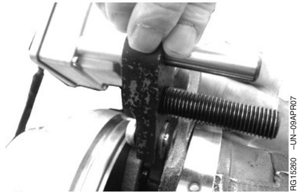
Position JDG10395 VGT Tool Base on Actuator Arm
