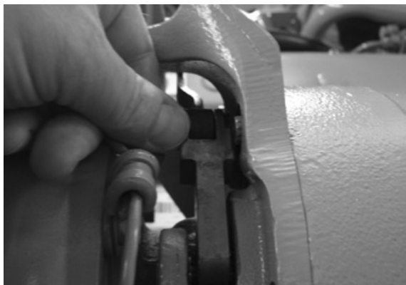
Check for Linkage Free Travel
