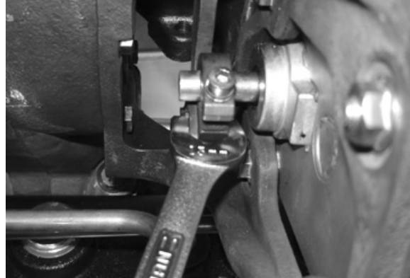
Using Wrench to Support Linkage
