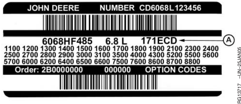
OEM Engine Option Code Label
