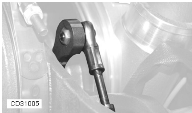
Actuator Linkage (Later design)
