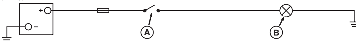
Locations of Circuit Malfunctions
