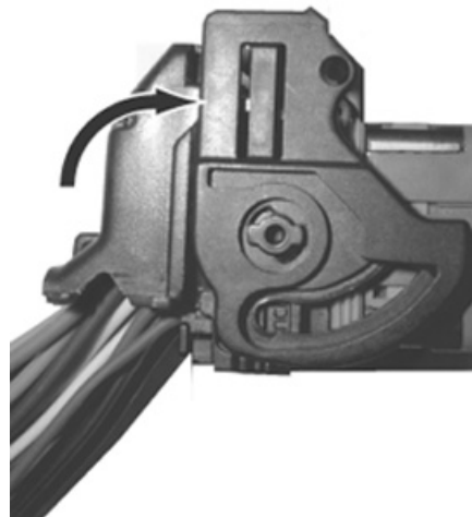
Rotate lock 90 Degrees
